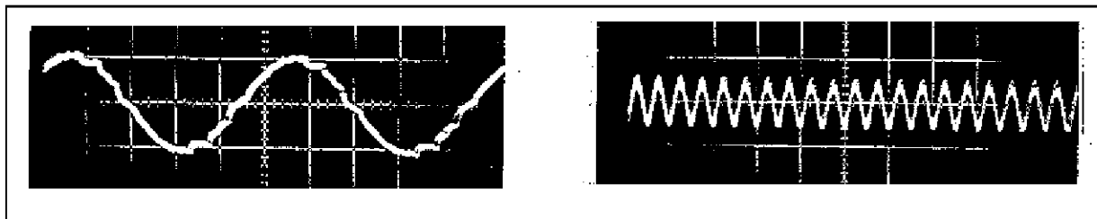
Figure 14. Current measured in motor phase
